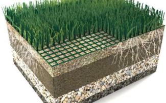
Hybrid Grass is basically a combination of synthetic grass and natural grass. Hybrid Grass is a natural grass reinforced by a combination of artificial turf fibers. FIFA accepts Hybrid Grass as Natural and classifies it as "Reinforced Natural Grass". This allows multi-functional use of their fields and offers extra benefits to clubs.
